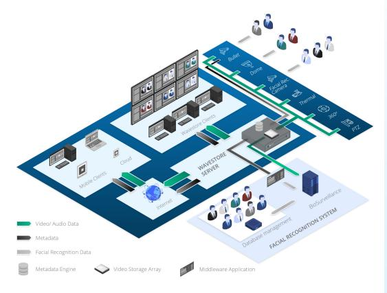
With the ability to pull all stored data related to a person, including name, number plate and phone number, Wavestore's metadata engine can be used to forensically search after an event. Furthermore, events can be triggered using the 'Cause and Effect' event rules engine, such as am alarm when a person of interest is detected.
